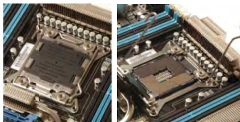
⊕ On the left is the unpacked CPU socket. You can open it by swinging open both left and right levers, and then the cover, to expose the CPU socket's very delicate array of contacts.
